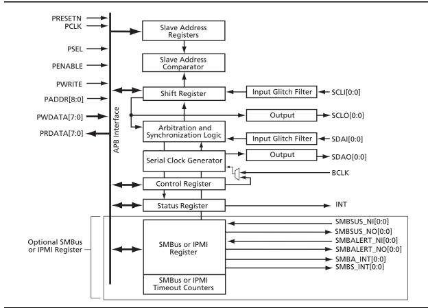
Figure 1-5 • Corel2C Block Diagram (single channel)
