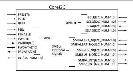
Figure 1-1 • Corel2C I/O Signal Diagram
