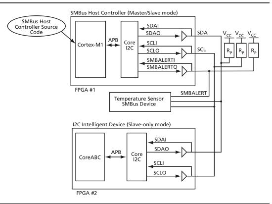
Figure 1 • CoreI2C SMBus Application Example
