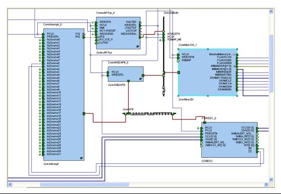
Figure 3-1 • Example System Using Cortex-M1 with Corel2C in a Two Channel Configuration
