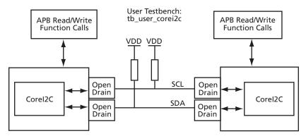
Figure 2-3 • Corel2C User Testbench
