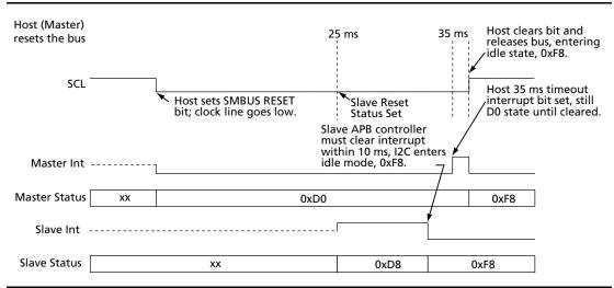
Figure 1-6 • SMBus Bus Reset Sequence
